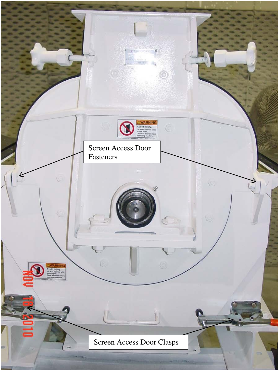
Figure 5-16: Removing the Screen Access Door
