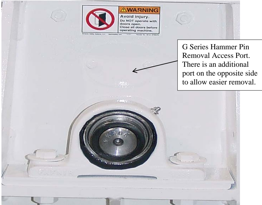
Figure 5-8: G Series Hammer Pin Removal Access Port
