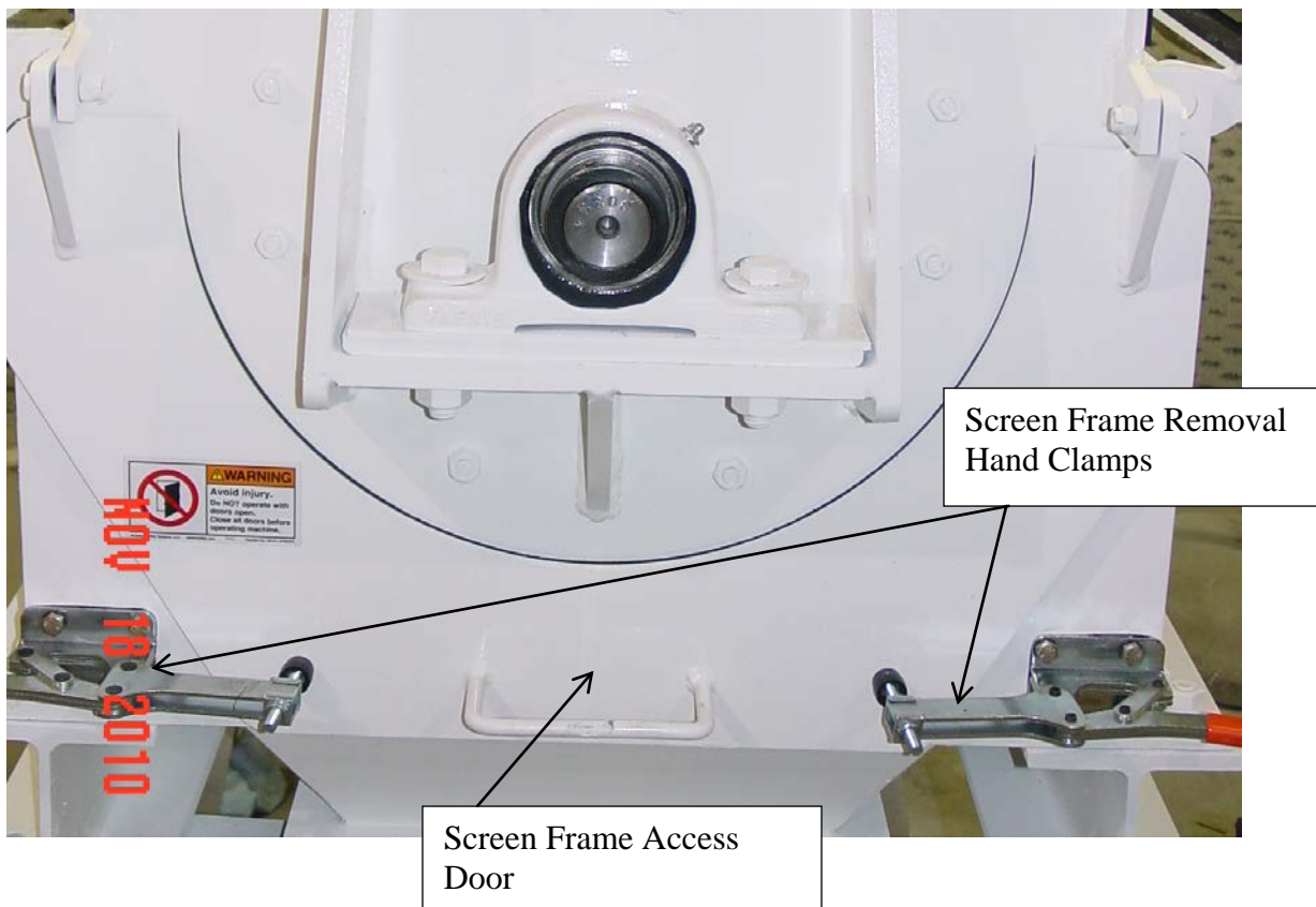
Figure 5-2: Screen Frame Access For G Series
