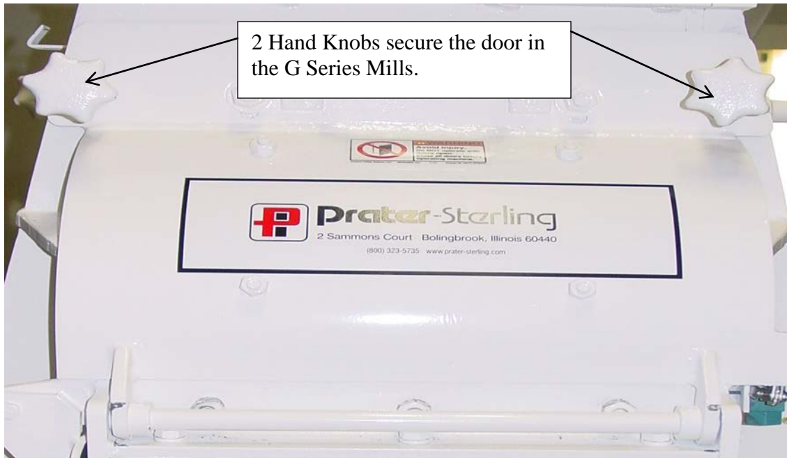
Figure 5-6: G Series Hammer Inspection/Replacement Access Door
