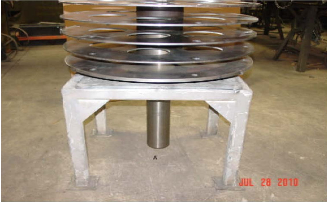
Figure 5-18: Rotor in stand for disassembly and reassembly
