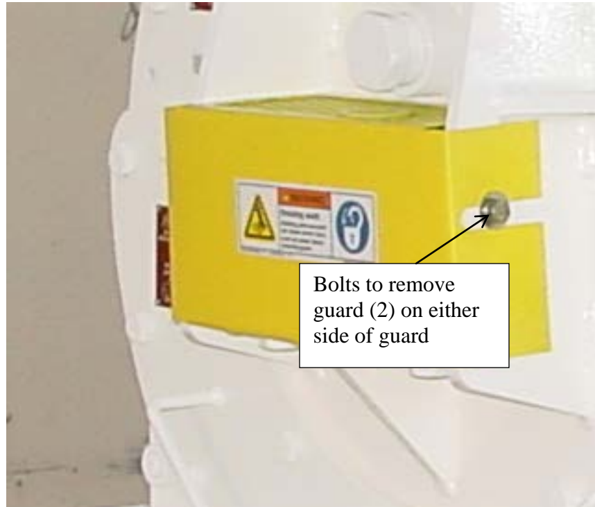
Figure 5-13: Non-Drive Side Bearing/Shaft Guard
