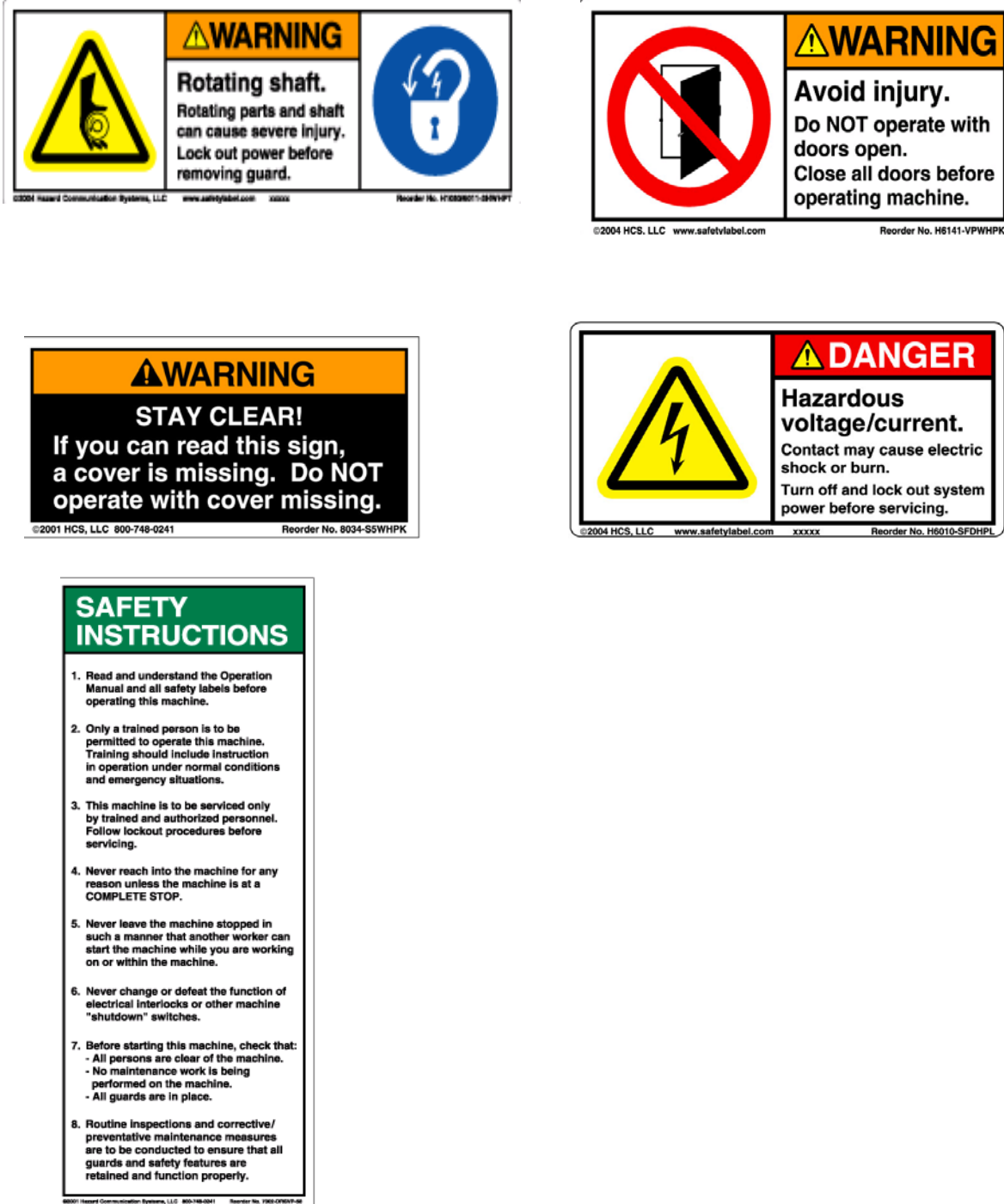
Figure 1-2: G Series Hammermill Safety Labels
